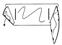
The side reflectors are attached to the lid next. There are two small 'L' shaped tabs on each side of the lid. Fold them back and insert them through the small slots on the wing reflectors, entering from the reflective side. The oven is now fully assembled.
